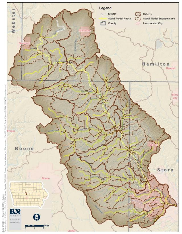
Figure 2-3. Watershed Model Drainage Areas and Stream Reaches
