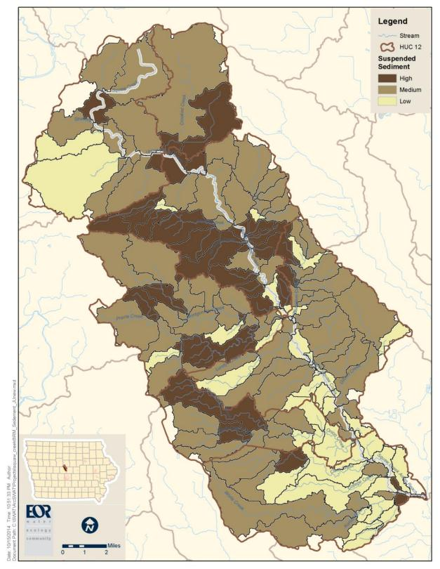
Figure 4-4. SWAT Model Sediment Load by Drainage Area (tons/acre per year)
