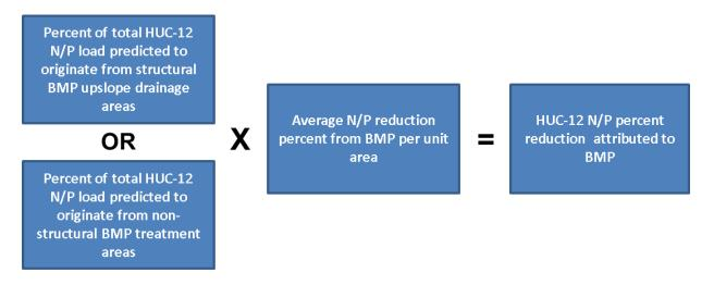
Figure 6-1. BMP scenario reduction analysis procedure for HUC-12 subwatersheds
