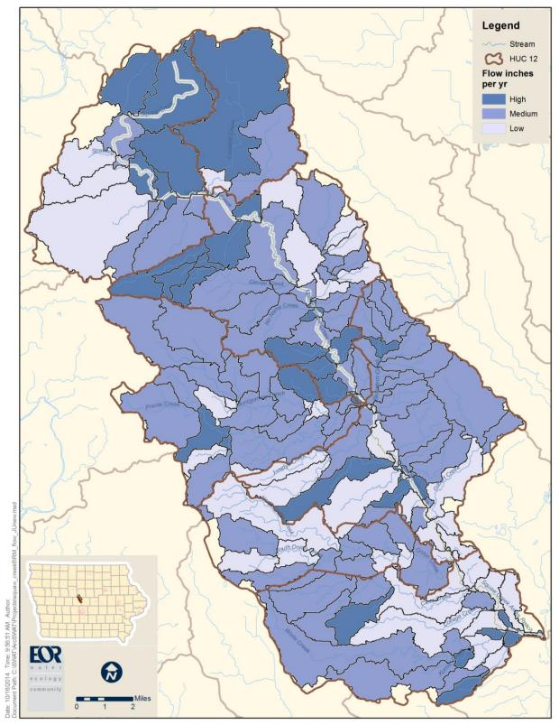
Figure 4-1. SWAT Model Flow by Drainage Area (inches/year)
