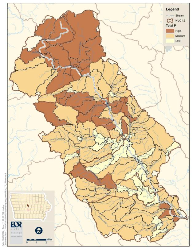
Figure 4-3. SWAT Model Phosphorus Load by Drainage Area (lbs/acre per year)
